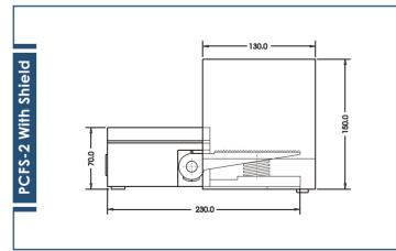
Foot Switches of heavy duty types are available i n two (Full down) or three (half down / full down) position operations.
