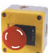
Mushroom Head Actuator 'Push Turn Type' with Legend - STOP, Contact - 1 'NC' for Stop
